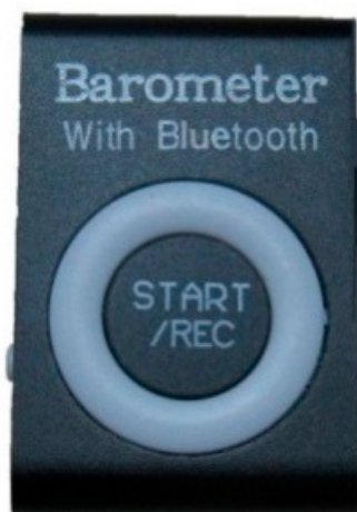
Figure 4. WTZ809A is a portal barometer with Bluetooth. It can work with Android smartphones or PCs though Bluetooth conjunction and can automatically measure, record, and send barometric pressure and temperature at a certain frequency.
