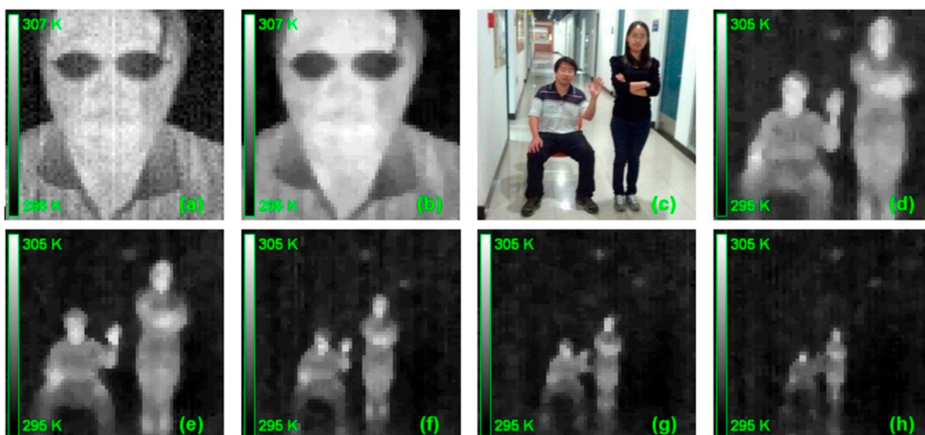
Figure 6. The performance of MTIS. (a) The raw thermal image of human face; (b) the corrected result of (a); (c) two people in different poses; and (d–h) the thermal image of (c) at 2, 3, 4, 5, and 6 m from the MTIS.
