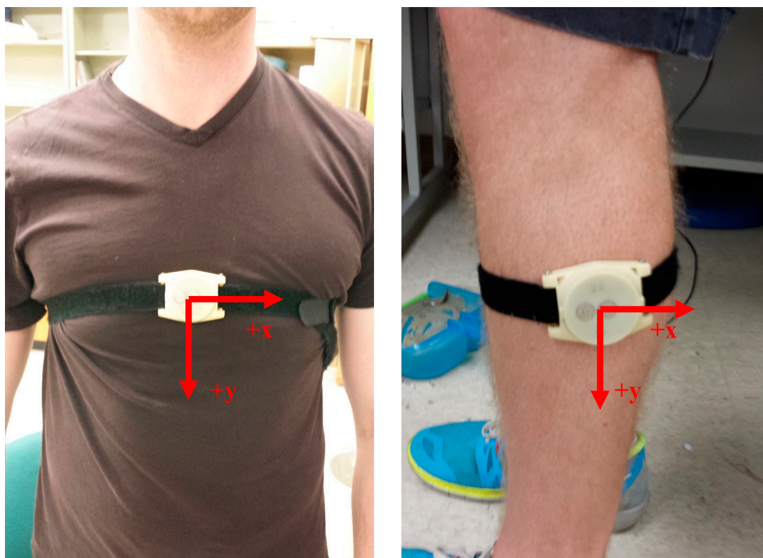
Figure 1. Example placement of the IMU's: over the sternum and laterally on the mid-shank. Each IMU was oriented using a left-hand coordinate system.
