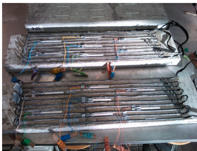
Figure 3. Bottom view of specimens SP1 and SP2—reinforced with Continuous Carbon Fibers Epoxy Composite.
