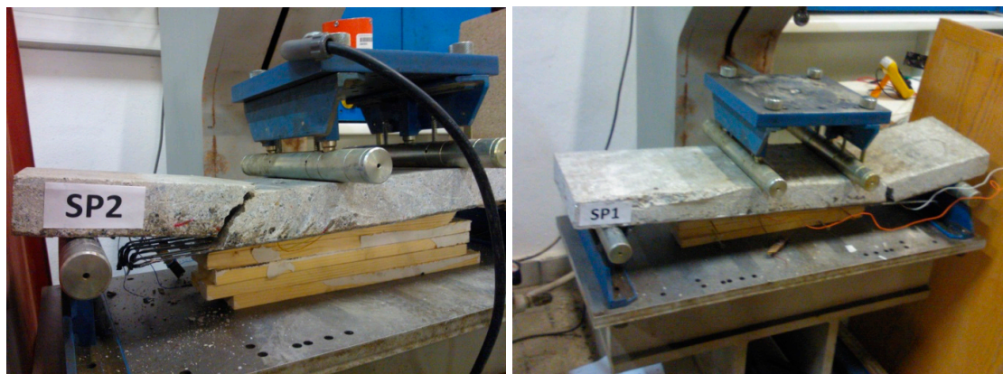
Figure 9. Damages and cracks for specimens SP2 and SP1.
