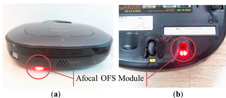
Figure 7. Vacuum-cleaning robot equipped with an afocal OFS module: (a) rear view and (b) bottom view.
