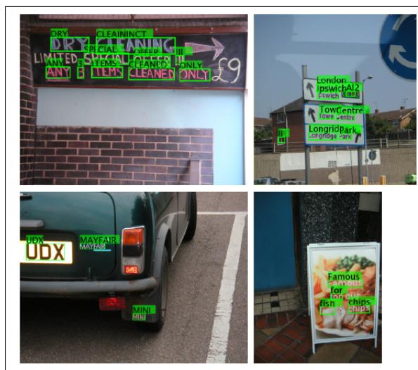
Figure 5. Optical character recognition in real time.
