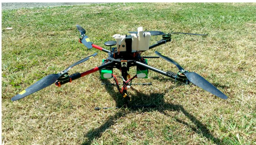
**Figure 5.** Quadcopter and modular gas-sensor system integrated.
