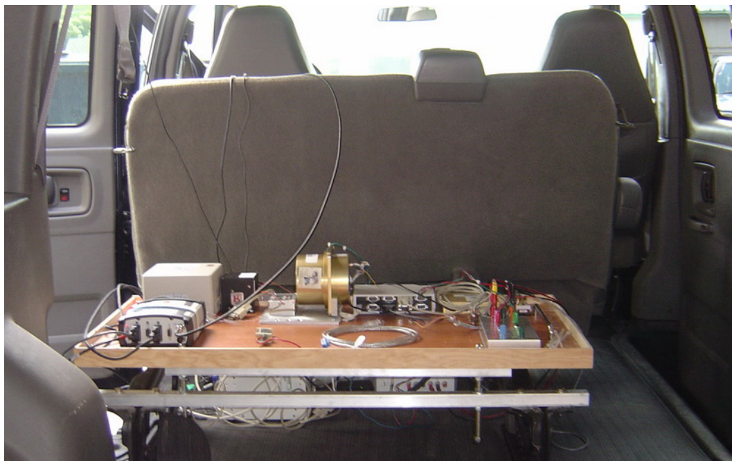
Figure 5. Navigation equipment and supporting hardware placed in a van for trajectory data collection.
