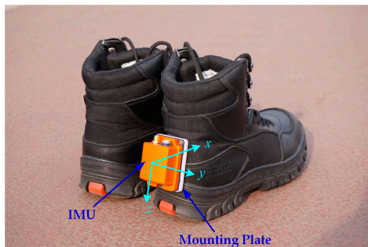
Figure 2. Pedestrian navigation shoe based on the IMU.
