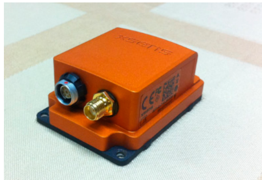
Figure 10. Xsens IMU for the foot-mounted PNS.
