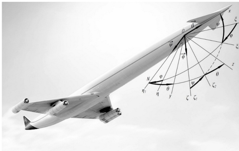
Figure 4. The scheme of the Euler angles ( \varphi : yaw angle; \psi : pitch angle; \theta : roll angle).
