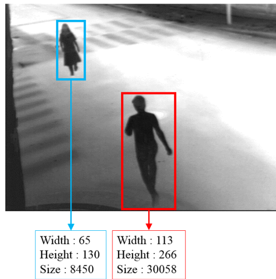
Figure 19. Example of different sizes of human areas because of camera viewing direction.
