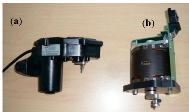
**Figure 2.** Indirect and direct drive actuator prototypes: (a), the indirect drive actuator, (b) the direct drive actuator. As presented in [7], both actuators are optimized with the same requirements in order to compare their energy consumptions.
