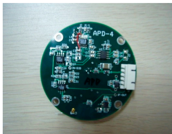
Figure 8. Implemented circuit for measuring the strength of the radiation of the reflective laser beam based on Figure 7.
