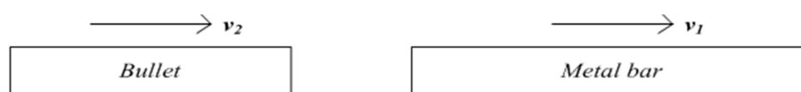
Figure 1. Coaxial impact of a limited elastic bar by a bullet and a metal bar.
