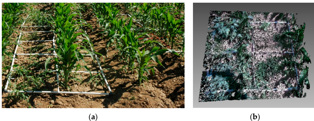
Figure 2. (a) Some frames located in the experimental field; (b) example of a mesh obtained with the Kinect v2 sensor.
