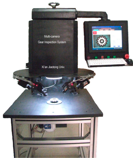
Figure 6. Prototype of multi-camera bevel gear inspection system.
