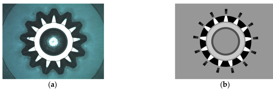
Figure 15. (a) Top surface of gear A 4 ; (b) The matching template.
