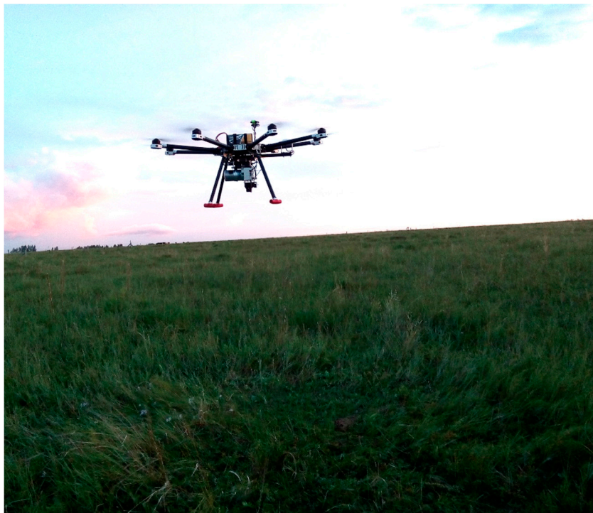
Figure 4. A ground-based photograph indicating the Li-Air fitted with Velodyne's HDL-32E lidar sensor.
