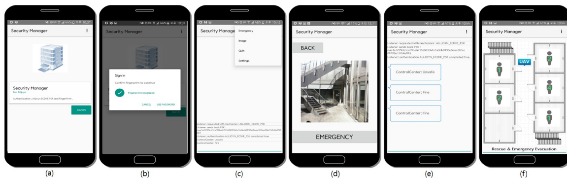
Figure 8. The interface of the building Security Manager app. (a) first page of security manager app, (b) fingerprint authentication process, (c) security manager app in a normal situation, (d) an abnormal temperature is detected, (e) security manager app in abnormal situation, (f) rescue and emergency evacuation mode of security manager app
