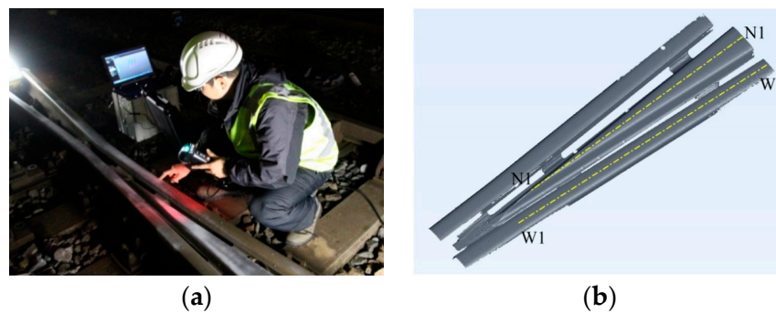
Figure 6. 3D profile measurement. (a) Measurement using HandyScan and (b) a measured 3D crossing profile. Cross sections W1 and N1 are along the centerlines of the wing rail and crossing nose, respectively.
