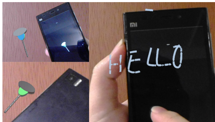
Figure A1. Virtual Probe controlled by the gyroscope located in the mobile phone. Remote drawing can also be achieved by drawing on the screen of the phone.
