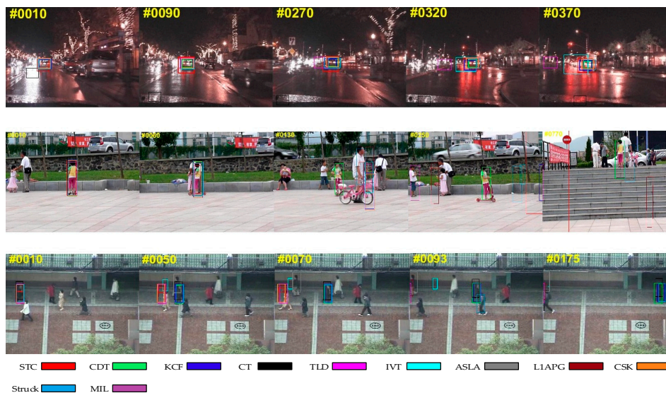
Figure 4. Qualitative results of our method and the nine state-of-the-art tracking methods on sequences Cardark , Girl2 and Subway . In these sequences, there is a background clutter problem.
