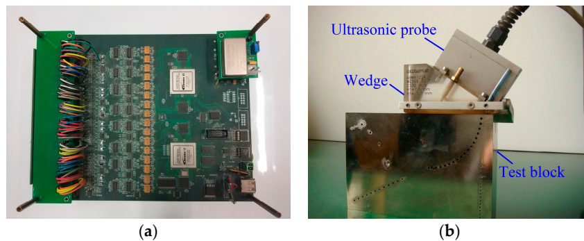
Figure 11. The ultrasonic phased array detection system. (a) Circuit board of ultrasonic transmitting and defect echo receiving; (b) Ultrasonic probe and standard test block.
