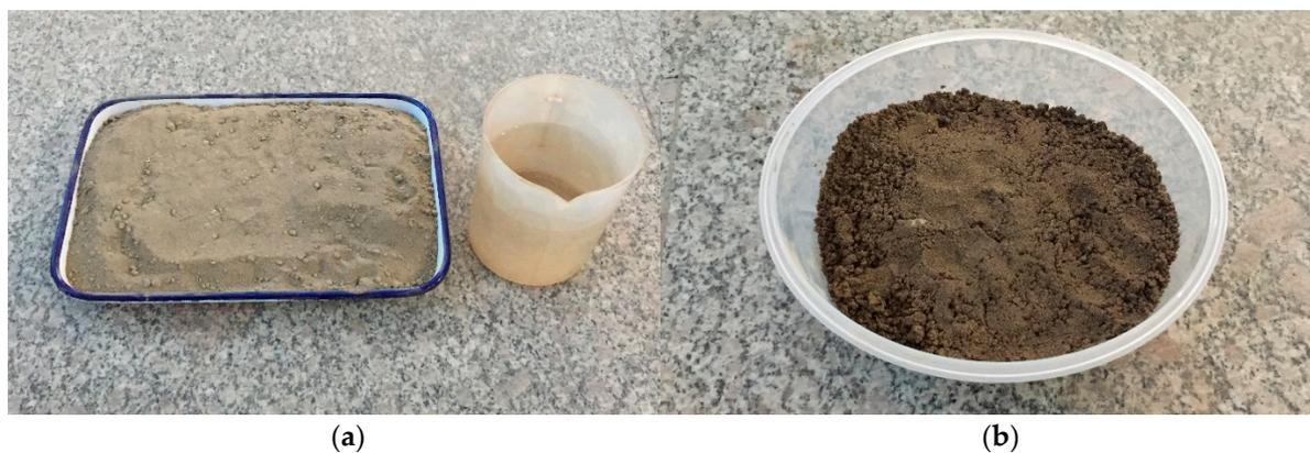
**Figure 2.** Preparation of the sandy soil. (a) Dry sand, (b) Sand soil (15% water content).
