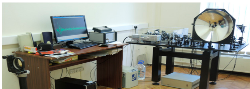
Figure 1. Experimental setup for THz signal measuring at long distance [38].
