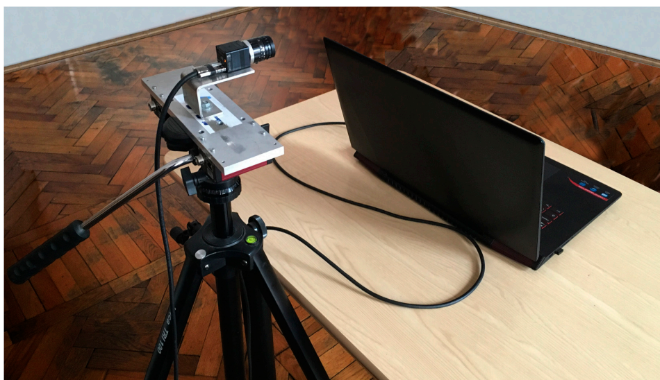
Figure 12. Physical system: the high speed Ximea camera is placed on a tripod and captures high temporal resolution frames of the subject.
