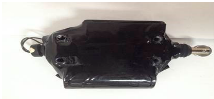
Figure 3. Detecting and communicating sensor of intelligent track skates.
