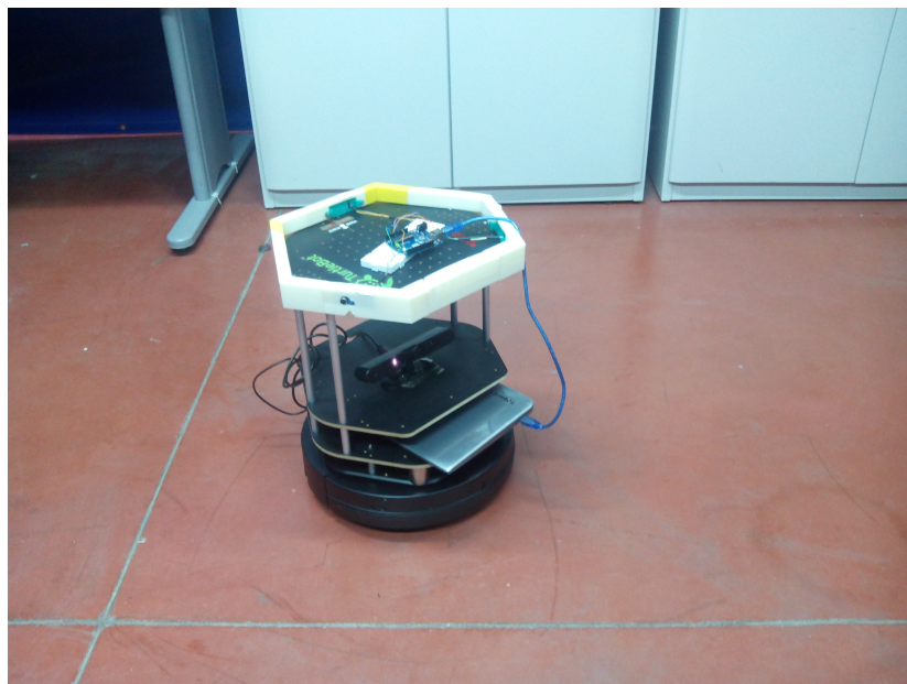
Figure 10. Turtlebot equipped with microphones and Asus 3D-sensor.
