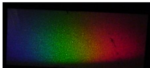
Figure 4. The spectrum given by the grism on ground glass. Its longer size is about 1 cm.
