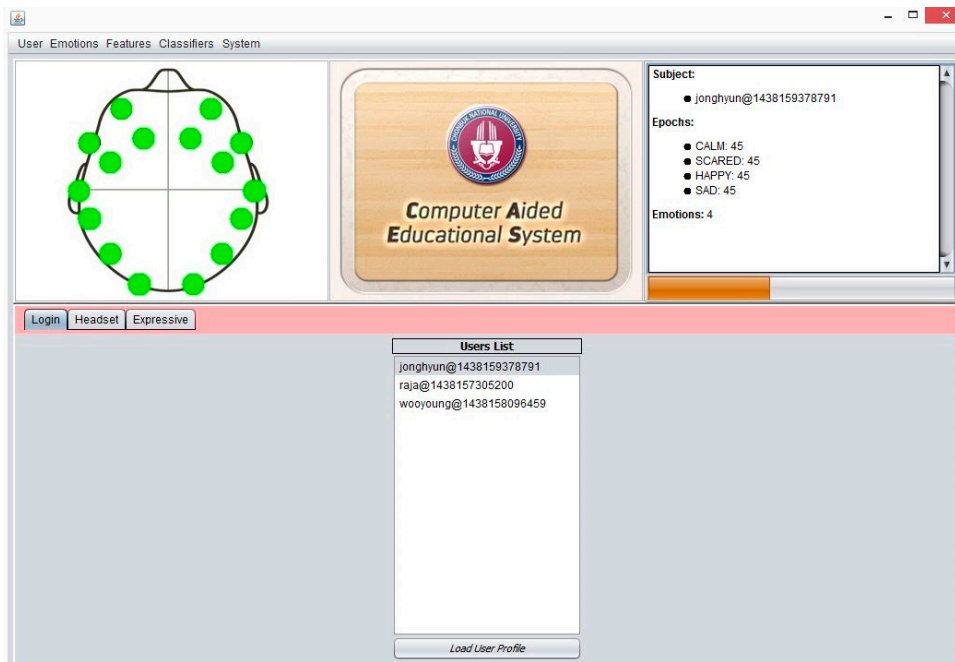
Figure 13. CAES (User Login); it provides the facility for users logging into the system. At this point the user can see the signal quality of the Emotiv headset channels, and the user can see the current user details such as name, epochs, etc.
