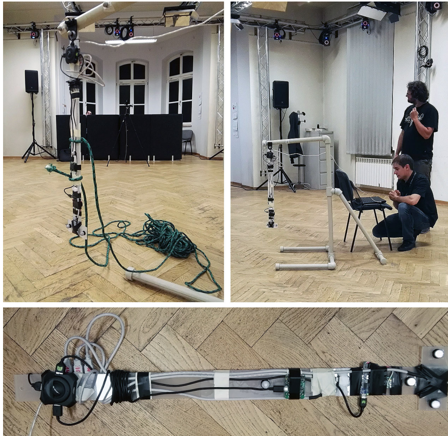
Figure 8. The pendulum with attached IMUs during the tests in the HML - motion capture laboratory.
