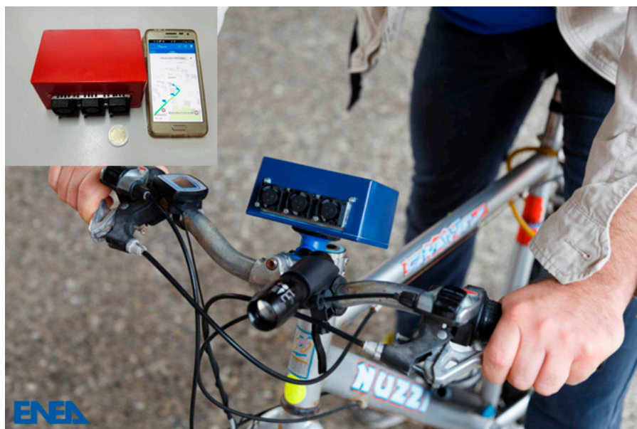
Figure 4. The Monica TM system is a solution for cooperative urban pollution monitoring [53]. It relies on an STM32 microprocessor and is equipped with an NO 2 , CO, RH, T and O 3 sensors. Data can be sent to a smartphone and shared with other users to construct a real-time pollution map of the city.
