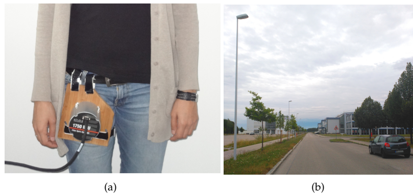
Figure 6. (a) The inertial data for the experiments analyzed in this section has been recorded with the IMU DSP-1750 attached to a wooden surface which is fastened to the leg, as if the sensor were introduced in the pocket. (b) Scenario of the experiments detailed in this section.
