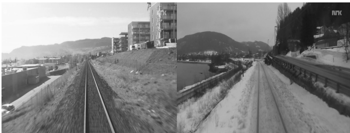
Figure 12. An example when the algorithm fails. The aliasing between the queried image (left side) and the image in memory returned by the algorithm is major.
