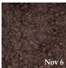
Figure 4. Original images for all soils at the beginning of the experiment (6 November 2014 images), after the first cycle of freezing–thawing followed by the biggest rain event (15 December 2014 images) and at the end of the experiment (10 February 2015 images). All soils experienced aggregate breakdown over time.
