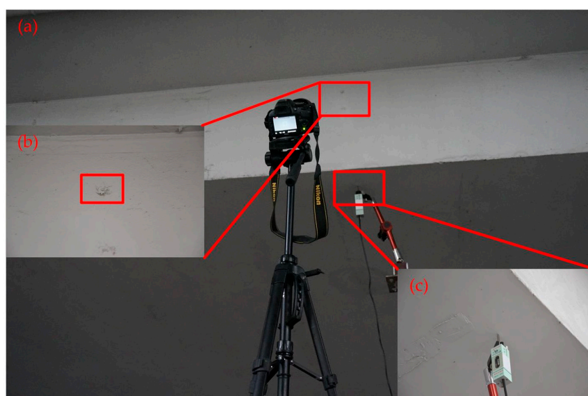
Figure 18. Field test: (a) Experiment environment; (b) Natural target; (c) Displacement by the STDS sensor.
