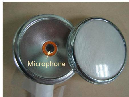
**Figure 2.** Each of the stethoscope head was made by encaving a condenser microphone into the bell taken from a conventional stethoscope.
