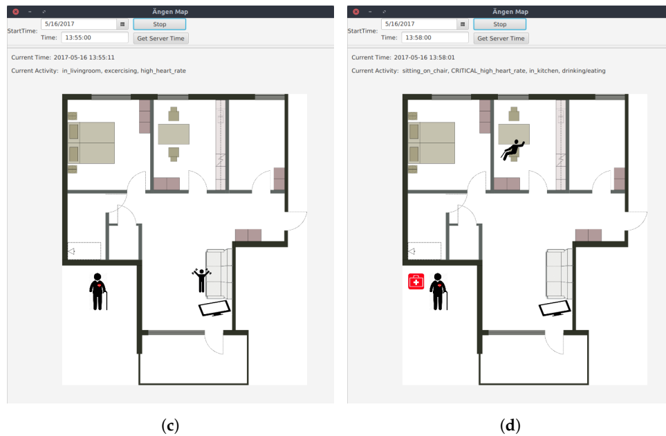
Figure 9. Time series signals from health and pressure sensor during the activities exercising and stress event . (a) The pressure and heart rate sensors during the exercising activity; (b) the pressure and heart rate sensors during the stress event; (c) recognized activities during the exercising activity; (d) recognized activities during the stress event.
