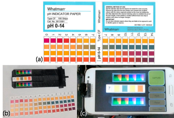
Figure 5. Preparations for calibration step: (a) Paper-printed comparison chart; (b) Split pieces; (c) Capturing the pieces on the mini light box.
