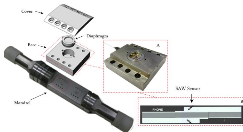
Figure 1. Pressure sensor assembly. In detail A : diaphragm mounted in the base. In detail B : top view of the SAW sensor.
