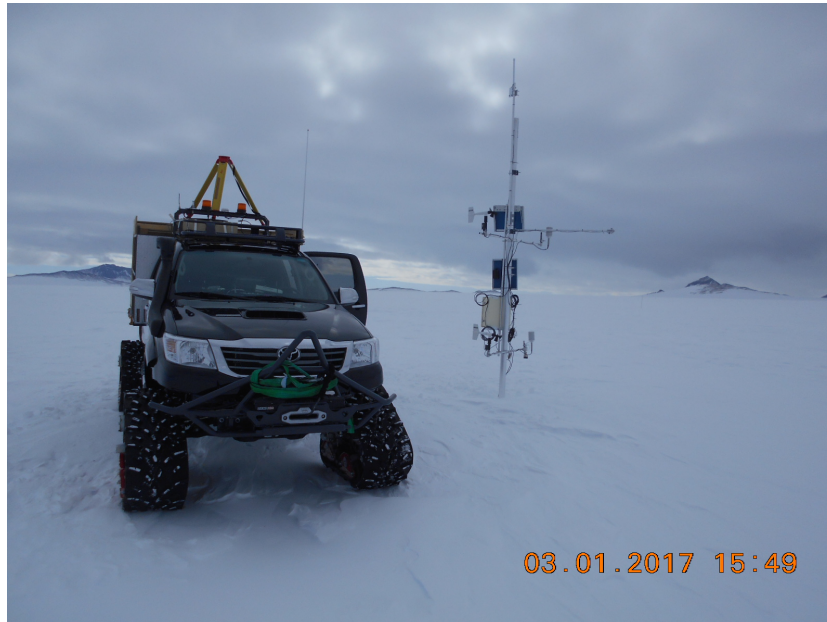
Figure 1. Mobile, carrying out the channel characterization experiments at one of the fixed wireless sensor nodes, monitoring meteorological conditions in the Antarctic.
