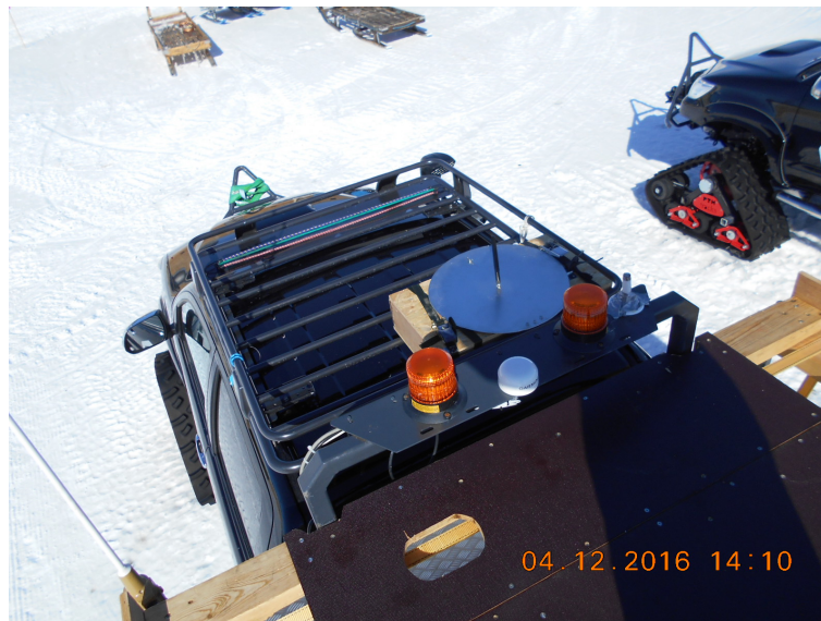
Figure 3. Detail of the 868 MHz antenna mounted on the 4 \times 4 vehicle.
