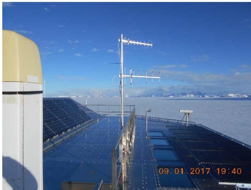
Figure 4. Fixed base station setup with directional antennas for the 434 and 868 MHz bands.
