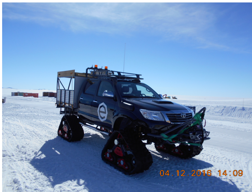
Figure 2. Mobile setup with omnidirectional antennas for the 434 and 868 MHz bands on the 4 \times 4 vehicle.
