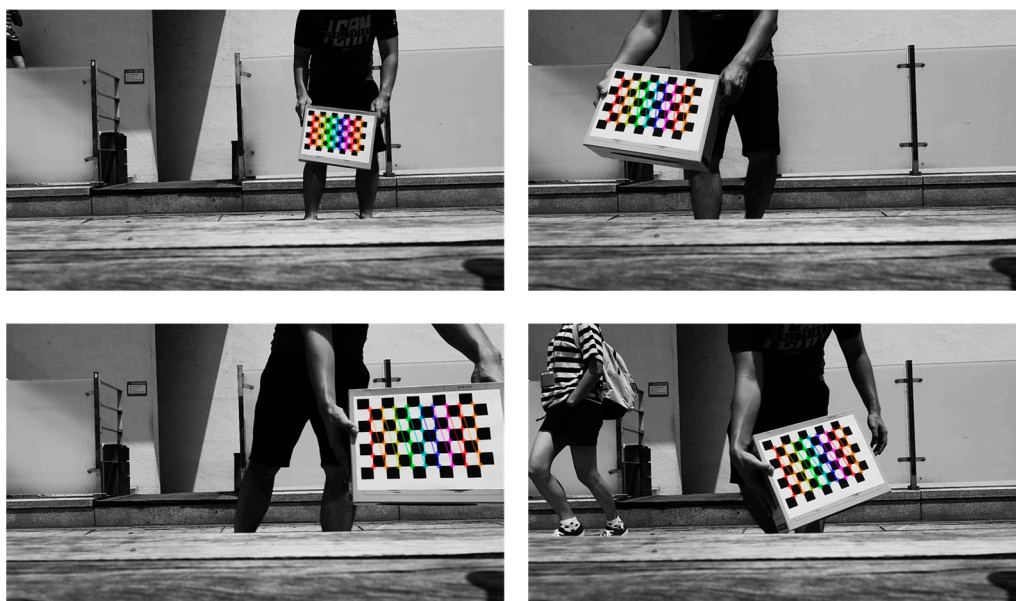
Figure 16. Some examples of our camera calibration process using chessboard pattern.
