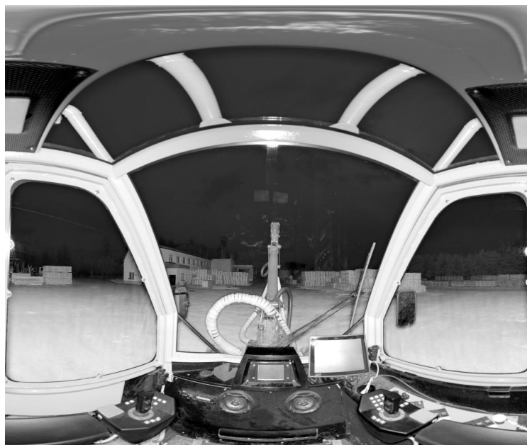
Figure 2. Driver's field of vision from harvester Model H50 Strojírna Novotný, Vitošov, Czech Republic (photo from scanner).
