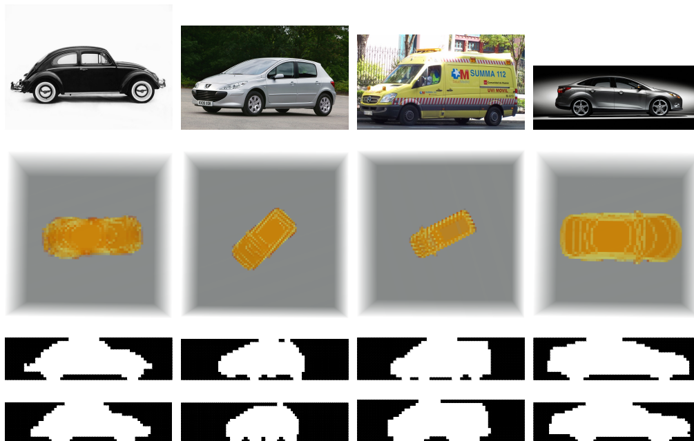
Figure 6. Results of tests on real images. In the first row, the original images as downloaded from the Internet. Second row, 3D objects rotated in the estimated angle and seen from above. Third row, projections after manually segmenting, centering and reducing the scale to 15 \times 60 pixels. Fourth row, projections generated applying the estimated rotation angle to the 3D model in the database.
