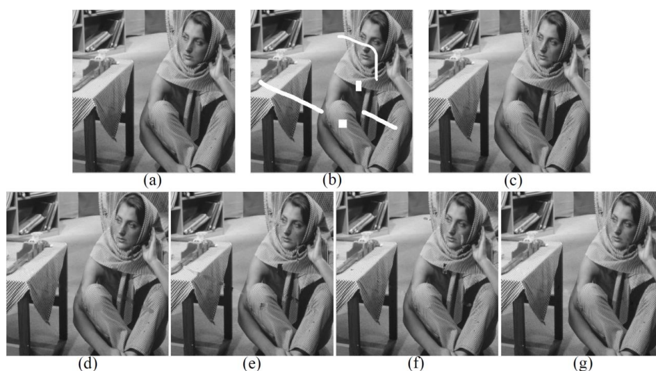
Figure 4. Comparison of Visual Effects on Barbara Image. (a) Original Image; (b) Corrupted Image; (c) Result of Ours; (d) Result of MRF; (e) Result of Texture Synthesis; (f) Result of [24]; (g) Result of MCA.
