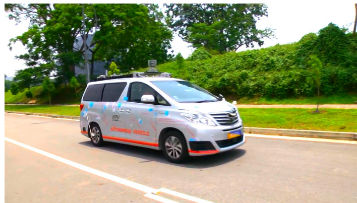
Figure 11. Autonomous vehicle equipped with GPS/IMU/DMI/LiDAR.
