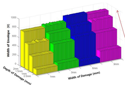
Figure 13. Variation of the width of envelope ( E_W ) according to the damage depth.
