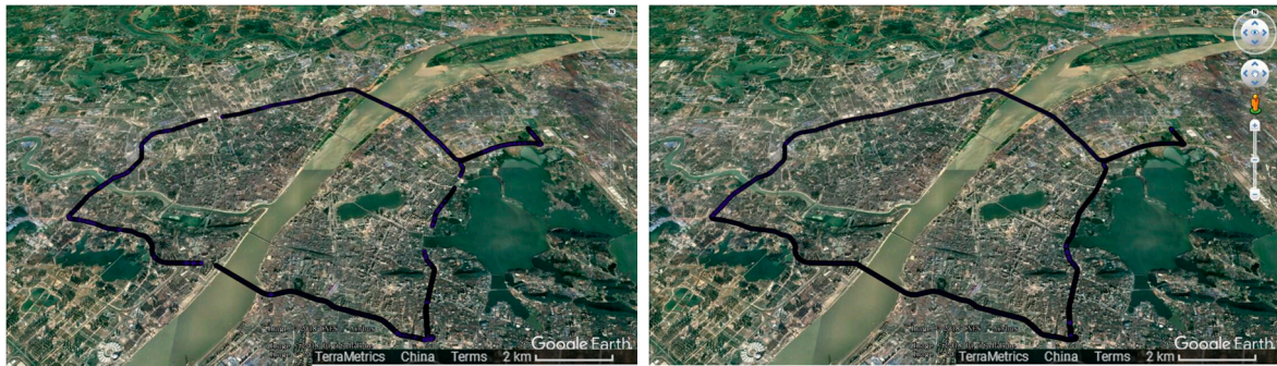
Figure 4. The whole vehicle trajectory on the 2nd Ring Rd; (The left one is obtained from GNSS, the right one is obtained from GNSS/INS).
