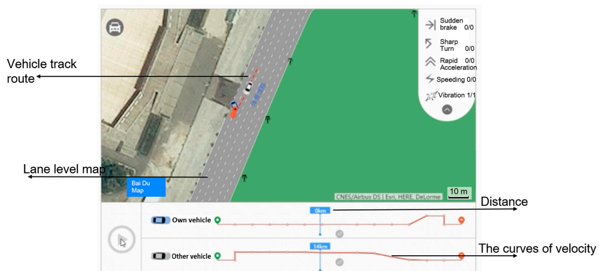
Figure 10. Reconstruction of the accident process.
