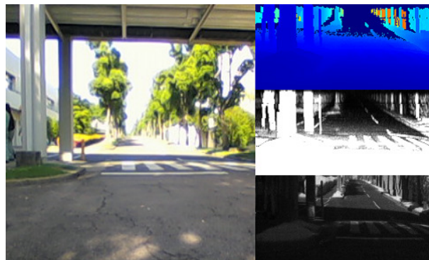
Figure 3. Examples of the output of the prototype LIDAR with the reference image in an outdoor environment: (right, top) range image data; (right, center) peak intensity image data; (right, bottom) monocular image data; (left) reference image captured by the camera.
