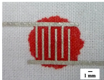
Figure 3. Photograph of the sensor after dropping 15 \mu\text{L} of blood.
