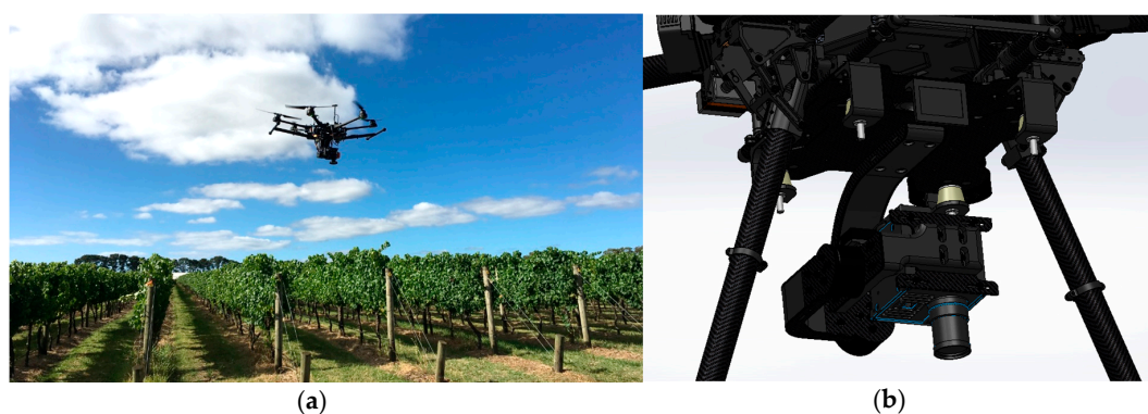
Figure 5. (a) Headwall Nano hyperspectral sensor on-board a S800 unmanned aerial vehicle (UAV); (b) Custom-made two-axis gimbal hosting the hyperspectral camera (SolidWorks 3D model).
